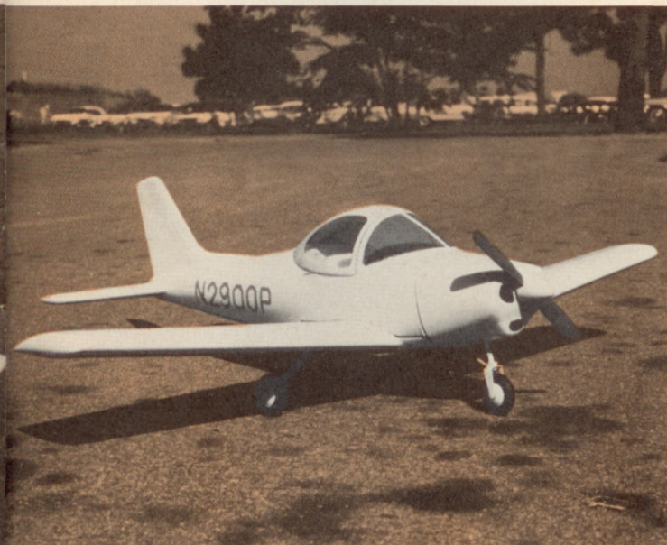
Fixed tricycle gear of plastic plane was designed with wide main tread in order to give extra landing and takeoff stability. Two-place " Papoose " has side-by-side seating and is powered by 108 h.p. Lycoming engine
